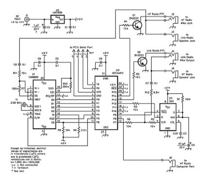
Figure 2—Schematic of the remote-base controller circuit. Equivalent parts can be substituted. Unless otherwise specified, resistors are <sup>1</sup>/<sub>4</sub> W, 5% tolerance carbon-composition or film units. Part numbers in parentheses are Radio Shack. Observe proper polarity for polarized components.
