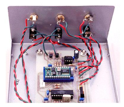
An inside view of the Remote-Base Station Controller. In this unit, a ZIF socket is used for U2 to allow easy replacement when experimenting.
